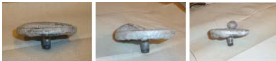
Figure 8. Solidified metal pool on the starting plate after the experiment. From left to right: Normal appearance, asymmetric metal, and formation of sphere.
